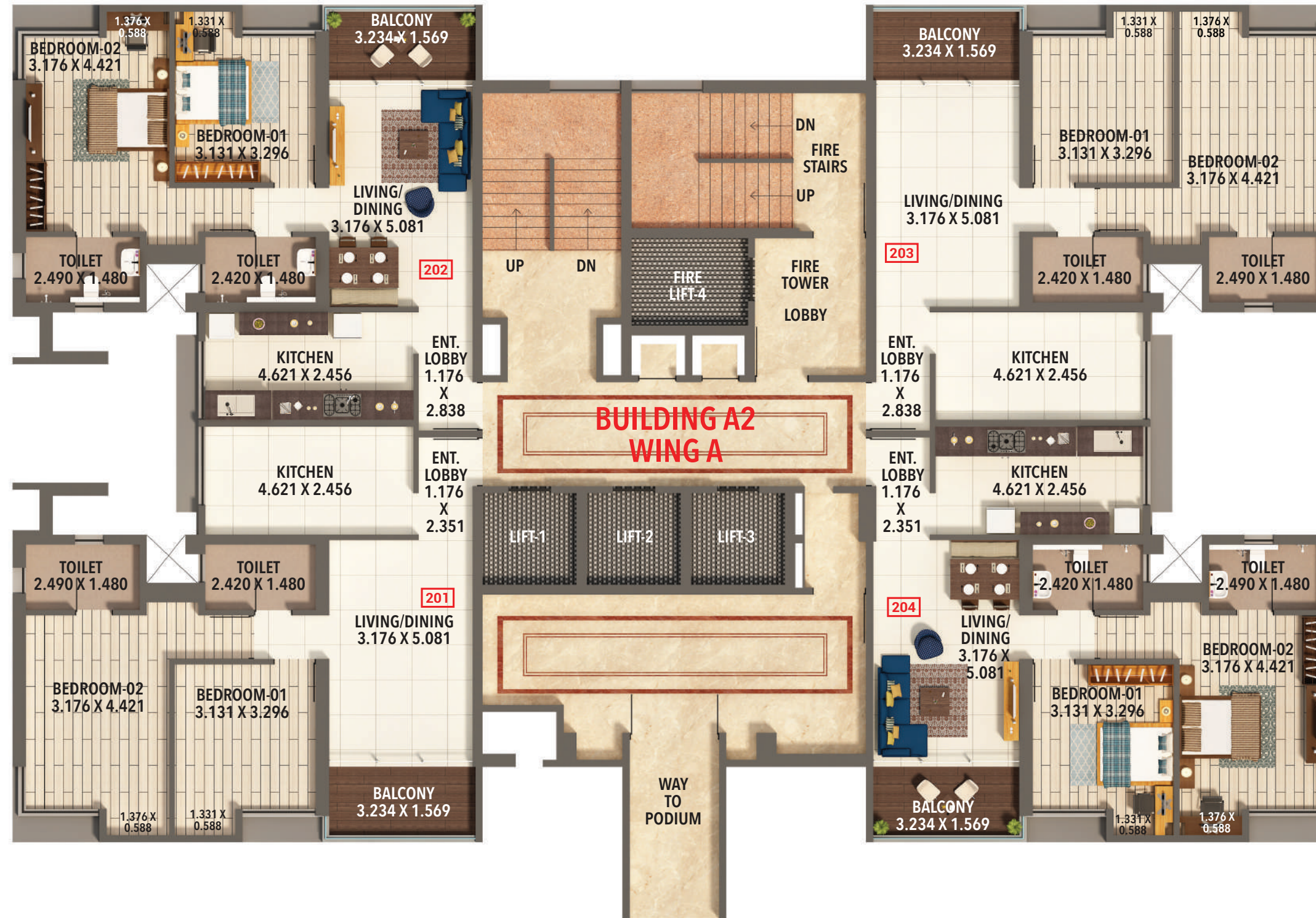
BUILDING A2 - WING A (AREA IN SQ.M.)
