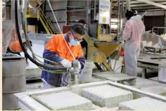
The application process for Spray-up GFRC is very similar to shotcrete in that the fluid concrete mixture is sprayed into the forms.
