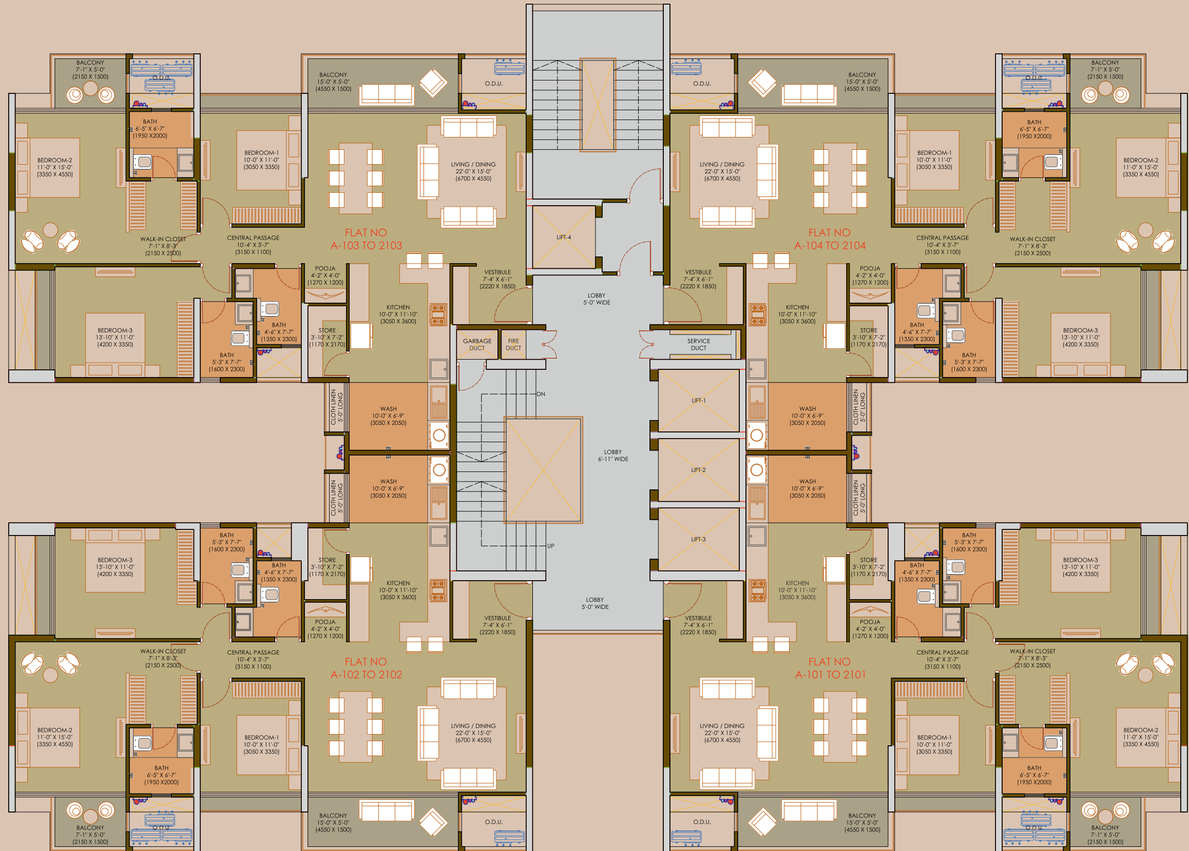
TYPICAL FLOOR PLAN (A -TOWER)
