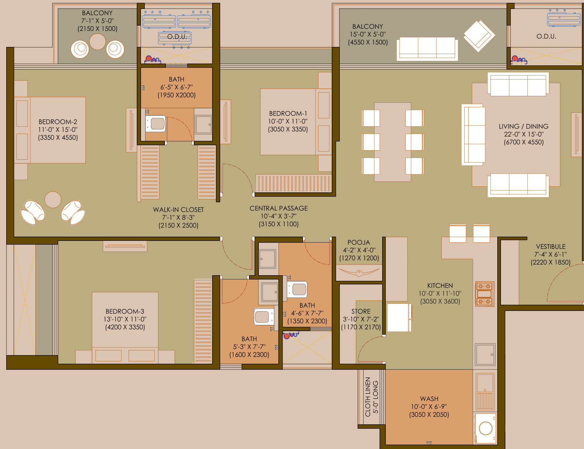
3 BHK UNIT TYPICAL FLOOR PLAN (A & B -TOWER)
