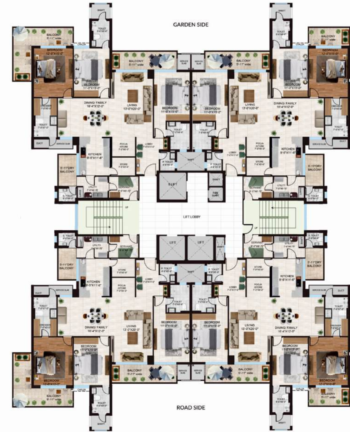
3BHK 2nd, 3rd, 4th, 5th, 10th, 11th, 12th, 13th Typical Floor Plan (End Tower)
