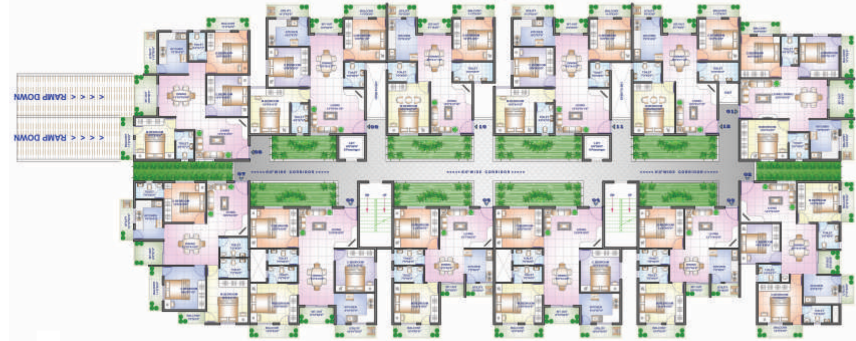
TYPICAL FLOOR PLAN COMBINATION OF 2 & 3BHK UNITS: 12units per floor 2BHK - SBA - 952sft & 1078sft, 3BHK - SBA - 1257sft to 1365sft
