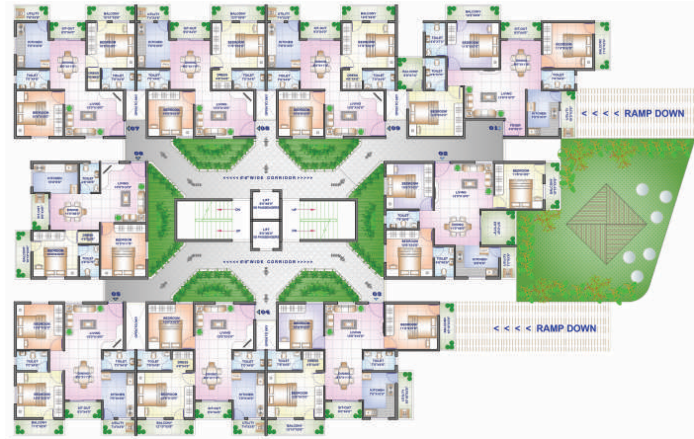
TYPICAL FLOOR PLAN COMBINATION OF 2 & 3BHK UNITS: 9units per floor 2BHK - 929sft to 1023sft, 3BHK - 1120, 1233 & 1357sft
