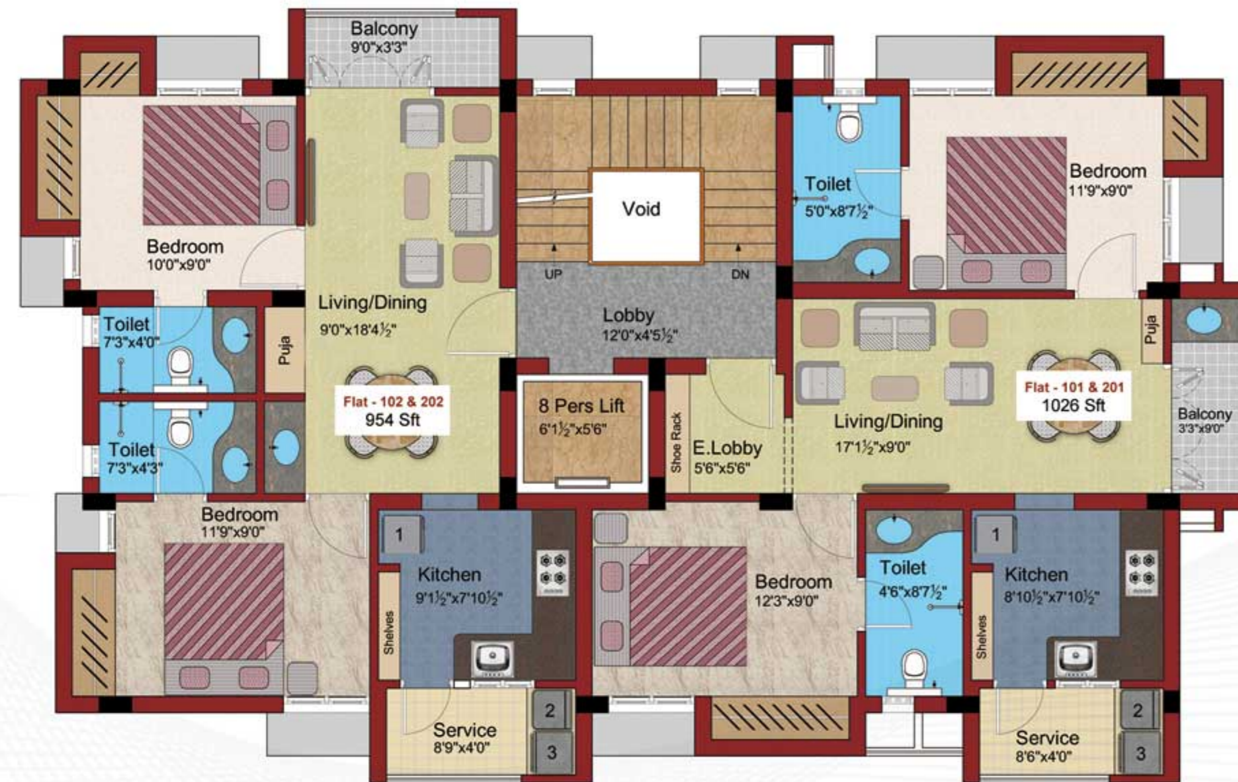
First and Second Floor Plan Block A
