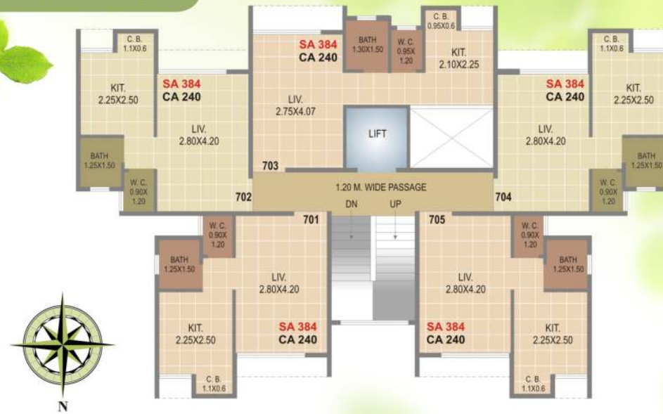
TYPICAL FLOOR PLAN FOR BLDG. NO. 6 & 7 (TYPE A)
