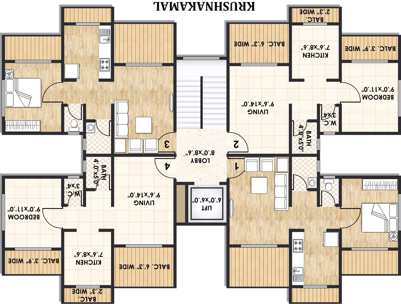
TYPICAL 1ST TO 5TH FLOOR PLAN OF BUILDING 3
