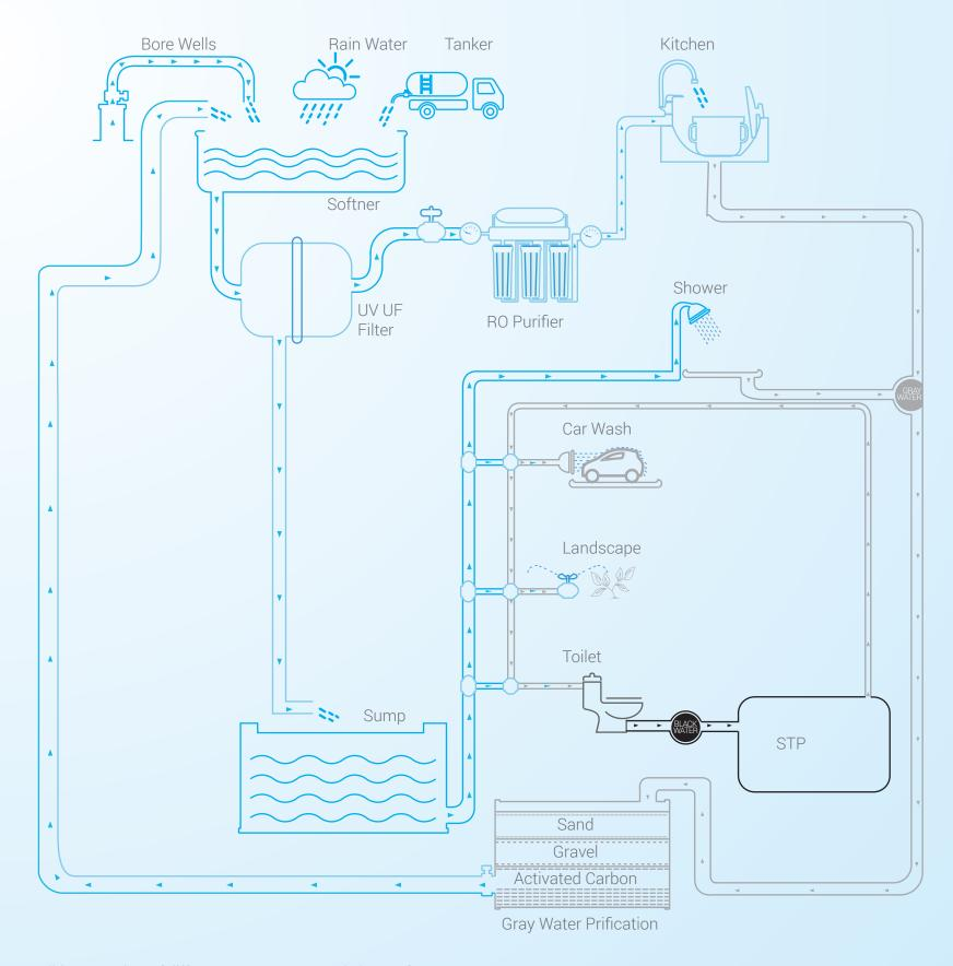
A central water softening plant conditions a variety of different water sources and pipes soft water to all taps. Drinking water is conditioned in a centralised RO and piped to every kitchen, reducing the cost and the need for any personal water purifier.
