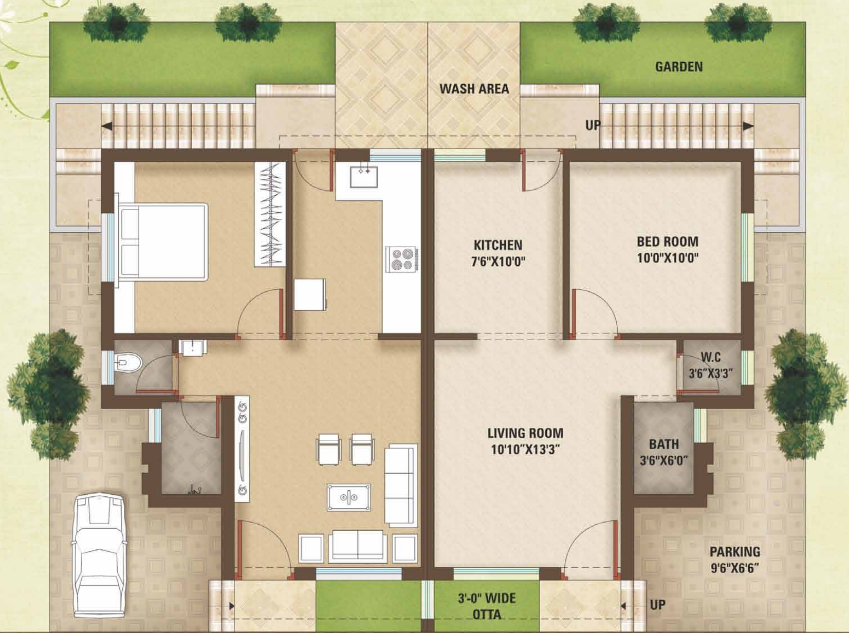
GROUND FLOOR PLAN PLOT AREA: 781. SQ.FT. SBA: 600. SQ.FT.
